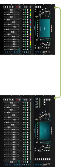
SQ to SQ direct 96kHz connection using gigaACE Send and receive all assignable I/O
