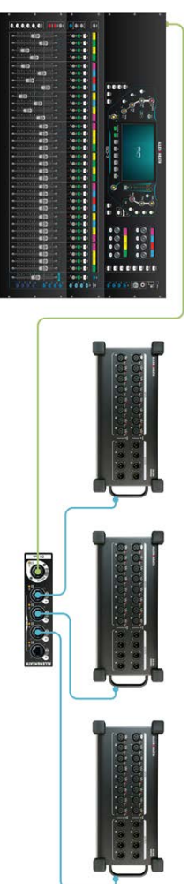
SQ expanded with 3x DX168s connected to a DX-Hub for full 96kHz operation, 48 remote inputs and 24 remote outputs
