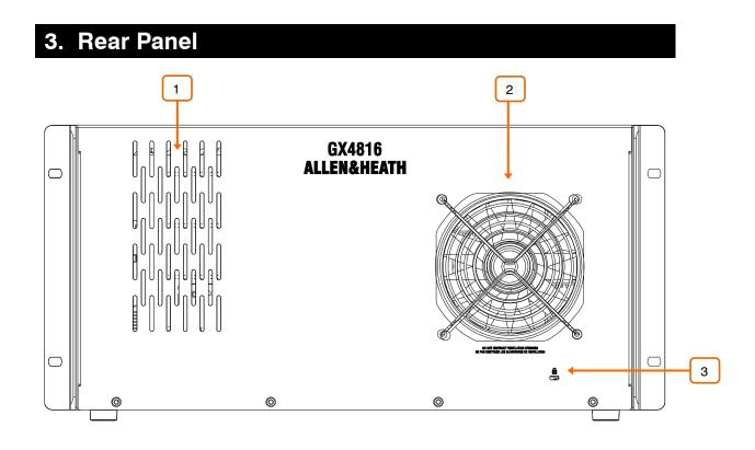
**Vents** – Ensure good ventilation and avoid obstruction of vents while operating. Avoid dirt or liquid ingress.
