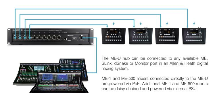
Multiple ME-U hubs can be daisy-chained together if more than 10 ports are required.
