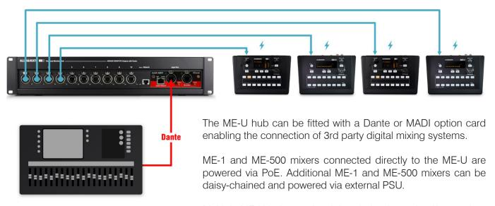
Multiple ME-U hubs can be daisy-chained together if more than 10 ports are required.
