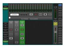
**Record Stereo or Multitrack** - Use the **Home** / **Qu-Drive** screen. Recording creates WAV files in Qu directories on the USB device. Stereo recording uses the same source as multitrack CH17 and 18.
