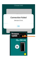
**Qu mixer not shown in Qu-Pad login list** – The mixer and router may have incompatible network addresses. Try a Network reset by pressing and holding the mixer recessed switch.
