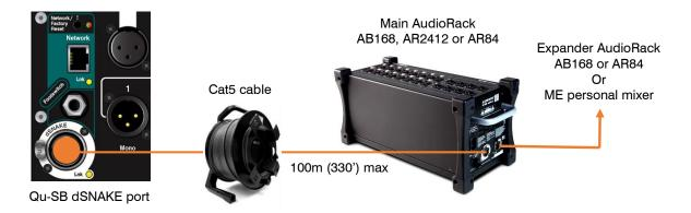
Plug into the AudioRack dSNAKE port. If you are connecting a second AudioRack connect it to the EXPANDER port of the first.
