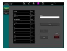
**To zero the board** as a start for setting up a new session or event you could use the Reset Mix Settings function on the **Scenes** page. This is a special Scene that resets all current mix parameters to factory default to give you a clear starting point to mix. It does not affect the memories and system settings and preferences.
