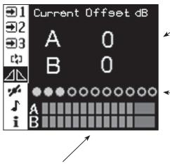
Loop Current bar graph for each channel. Shows Loop output current in 2dB steps from >-20dB to 0dB in green. Red = clipping
