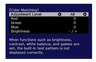
6. Press the left or right arrow buttons to select a value for the **Adjustment Level** setting.
