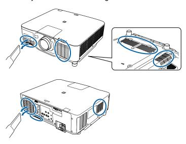
**Caution:** Do not use canned air. The gases may leave a flammable residue or push dust and debris into the projector's optics or other sensitive areas.
