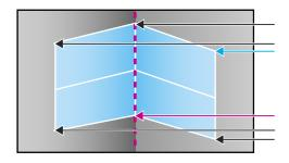
• For vertical corners, adjust the left and right areas using the points nearest the center of the image as your reference points.
