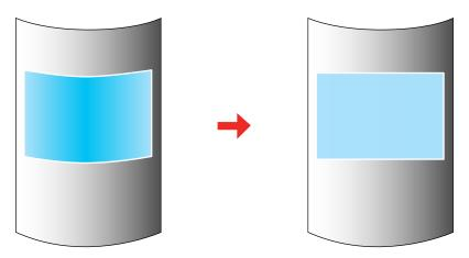
**Note:** For the best results, keep the lens centered using lens shift. The image may not be evenly focused throughout even after performing the steps here.
