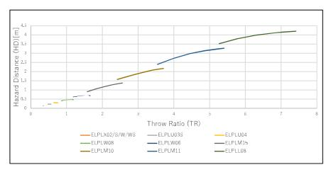
The installer and users of this projector must understand the risk and apply protective measures based upon the hazard distance as indicated in this user guide. Installation method, separation height, barriers, detection systems or other applicable control measures shall prevent hazardous eye access to the radiation within the hazard distance. See IEC Standard 62471-5: 2015 for additional guidance.
