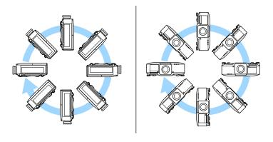
If you project from the ceiling or from the rear, select the correct **Projection** setting and, if necessary, adjust the **OSD Rotation** setting.
