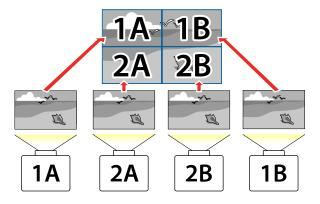
**Note:** Before tiling, make sure the displayed images from your projectors are rectangular, correctly sized, and focused.
