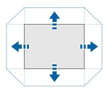
The distance the image can be shifted varies depending on the installed lens. The limits are described in the following table. You can shift the image up to the listed percentage of the image height or width.
