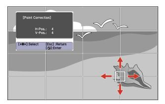
10. Press the arrow buttons to correct the image shape in all necessary directions.
