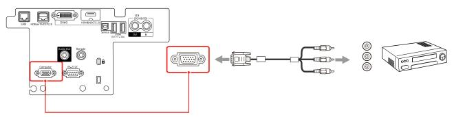
3. Tighten the screws on the VGA connector.
