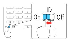
3. Press and release the **ID** button. Within 5 seconds, use the numeric buttons to enter a number for the projector (for example, **1** for projector ID 1).
