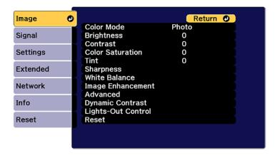
4. To automatically adjust the amount of light based on the brightness of the image, select the **Dynamic Contrast** setting and press **← Enter**. Choose from the following options:
