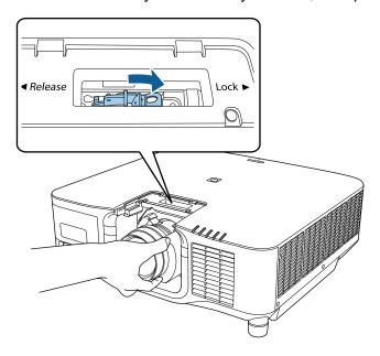
**Note:** Make sure the lens is securely attached.
