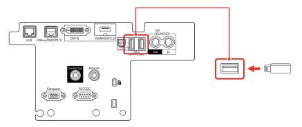
**Note:** Connect the flash drive directly to the projector. Do not use a hub or your settings may not be saved correctly.
