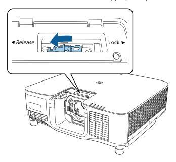
3. Insert the lens straight into the projector's lens socket with the white dot facing up.
