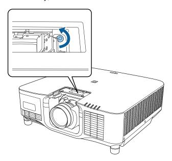
5. Hold the lens firmly as you pinch the lock lever and move it to the **Release** position.
