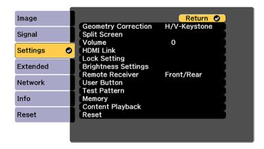
4. Select the **Geometry Correction** setting and press **← Enter**.
