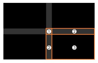
**Note:** The area you selected is displayed in orange. Adjust overlapping areas starting with the brightest areas first. For example, adjust area 2 to match area 1, then adjust area 3 to match area 2.
