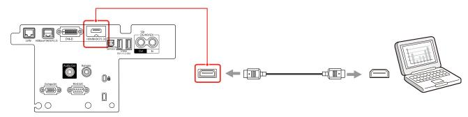
**Note:** The projector converts the digital audio signal sent from your computer into a mono analog signal for the internal speaker or a stereo analog signal if you are connecting to external speakers. (Make sure the HDMI audio playback device on your computer's audio settings is set to **EPSON PJ**.)
