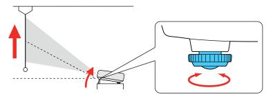
3. If the image is tilted, rotate the front and rear feet to adjust their height.
