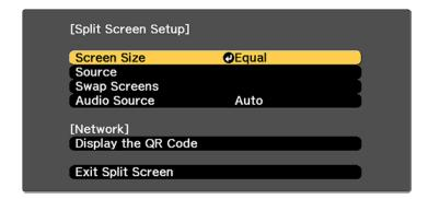
3. To select an input source for the other image, select the **Source** setting, press **✓ Enter**, select the input source, select **Execute**, and press **✓ Enter**. (You can also change image sources, if necessary.)
