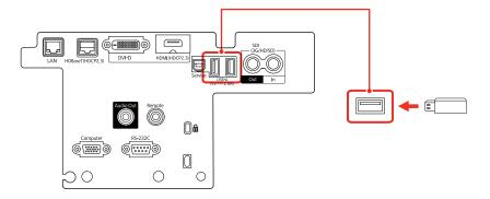
**Note:** Connect the flash drive directly to the projector. Do not use a hub or your settings may not be saved correctly.
