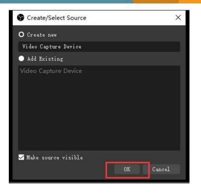
Step2. Right-click "Video Capture Device" and select properties, enter the properties interface, and select the signal source as your device. Users can set other parameter setting in the properties pages and then click OK.
