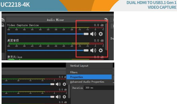
Step4. Enter "Advanced Audio properties" can change the setting about the volume, balance, audio monitoring, and Tracks etc.
