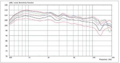
0/10/20/30/40/50 degree off-axis measurements of CDD15 (wide-axis).
